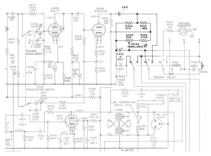
Removing Record-Noise Balance circuit from Ampex 300, 400, and 350 recorders / 2018 August 10
