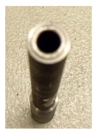
5) Bearing installation requires a special bearing pusher. This can be machined from a piece of cold-rolled steel. The most critical requirement is that it be carefully drilled and then reamed to **8mm ID at a depth of 4 inches**.
