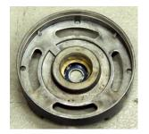
7) Place rotor back in the motor housing with the rounded (long) end up. You may need to heat the lower end bell slightly to permit easier installation.
