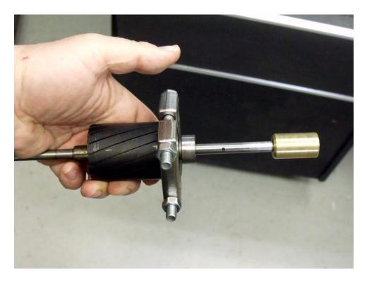
3) After removing brake drum and turntable from the rotor rotor, remove the die-cast support plate. Then mark the orientation of the upper motor end bell by scratching across the junction between the end bell and the motor housing (you do not need to remove the lower end bell).
